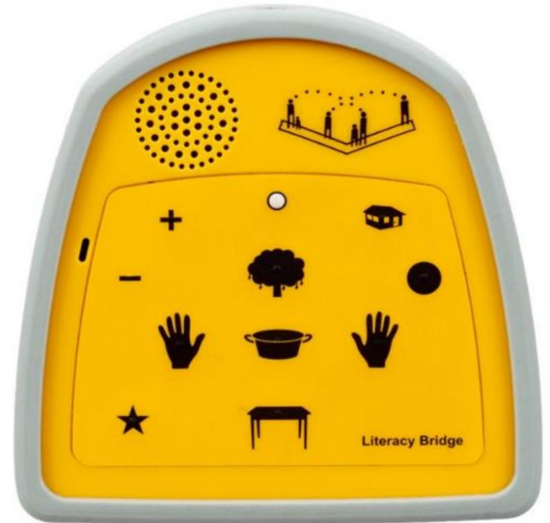
Figure 1: The Talking Book showing the icons of the new UI design using PD.
